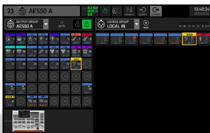
- Source LCL 7 is routed to out AES50-A ch23
